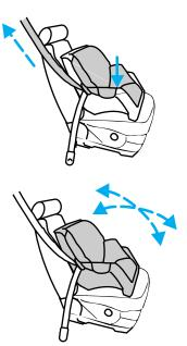
10. Try to pull the belt out of the retractor to make sure the retractor is in the automatic locking mode (you should not be able to pull more belt out). If the retractor is not locked, unbuckle the belt and repeat steps two through nine.
